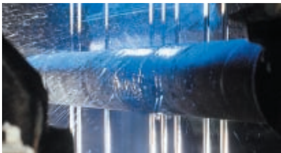
Galvanising of wire
