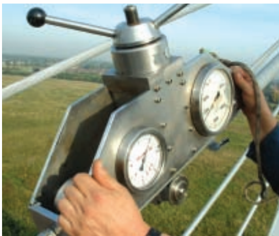
Strand tension measurement
