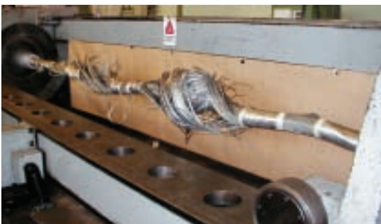
Strand breaking load test
