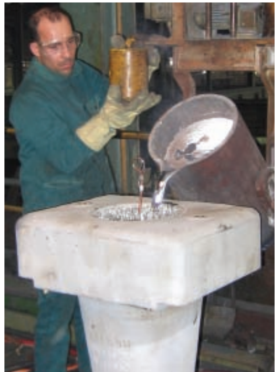
Filling of socket with zinc alloy
