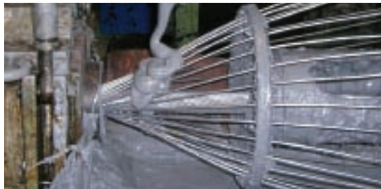
Application of spinning compound
