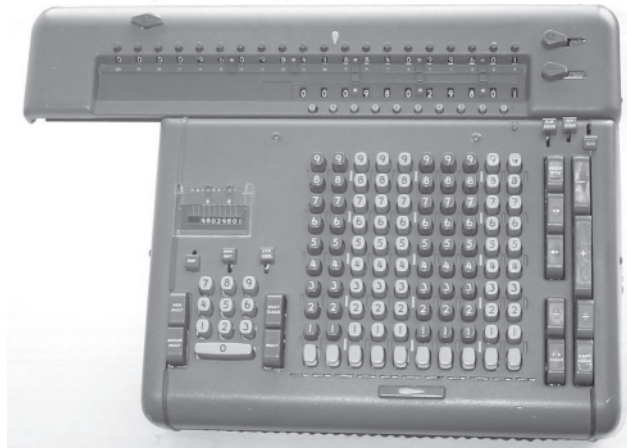
Collection of the author Friden automatic electromechanical calculator
