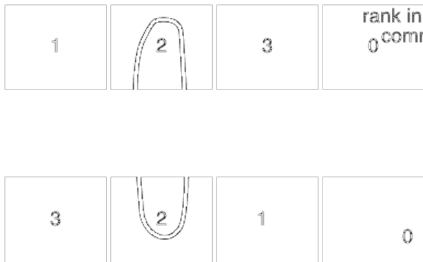
Figure 7.2: Illustration of ranks in an intercommunicator setup
