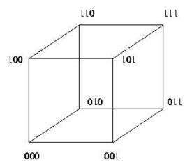
It is sometimes helpful to build up a cube from the lower-dimensional cases. To build a (d+1)-dimensional cube from two d-dimensional cubes, just follow this recipe:
