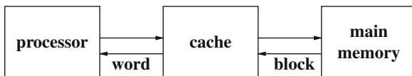
Fig. 2.32 Data transport between cache and main memory is done by the transfer of memory blocks comprising several words whereas the processor accesses single words in the cache
