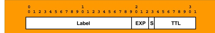
Label = 20 bits COS/EXP = Class of Service, 3 bits S = Bottom of Stack, 1 bit TTL = Time to Live, 8 bits
