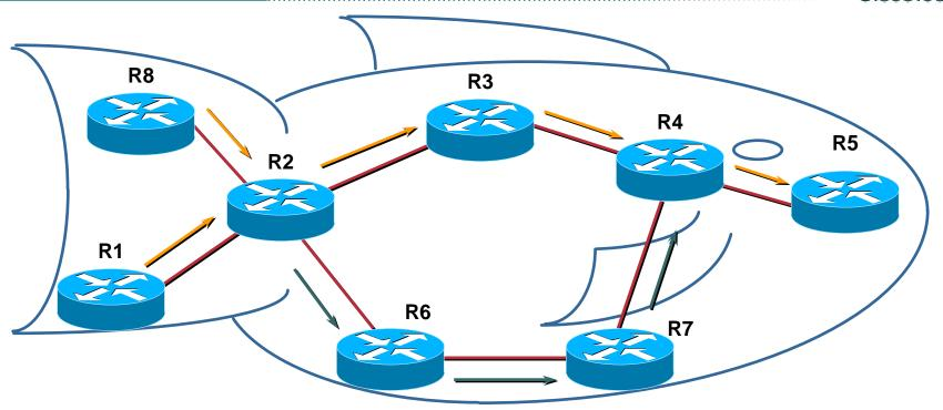
IP (Mostly) Uses Destination-Based Least-Cost Routing Flows from R8 and R1 Merge at R2 and Become Indistinguishable From R2, Traffic to R3, R4, R5 Use Upper Route
