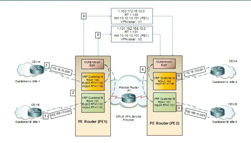
• The import route target is associated with each VRF and identifies the VPN v4 routes to be imported into the VRF for the specific customer.
