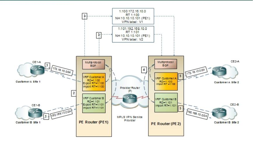
• When a VPN route learned from a CE router is injected into VPNv4 BGP, a list of VPN route target extended community attributes is associated with it.
