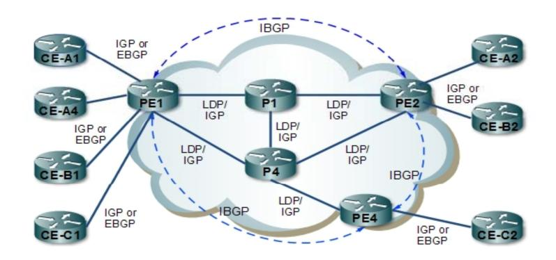
• The only requirement on the CE router is a routing protocol or a static route that enables the router to exchange IPv4 routing information with the connected PE router.
