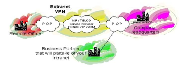
An example of an extranet is a company that has outsourced its help desk functions and sets up a VPN to provide a secure connection from its corporate office to the outsourcing company.
