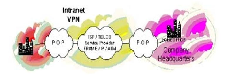
An example of intranet VPN is the connections between different locations within a company's infrastructure, such as VPNs between two offices
