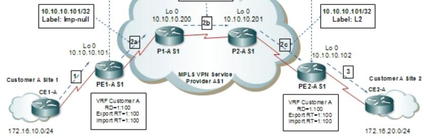
2a. Edge LSR PE2-AS1 requests a label for the 10.10.10.101/32 prefix using LDP from LSR P2-AS1 then from P1-AS1 then from Edge LSR PE1-AS1. Edge LSR PE1-AS1 allocates a label of implicit-null and sends it to P1-AS1.
