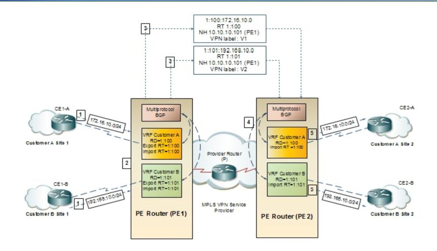
• The export route target is appended to a customer prefix when it is converted to a VPNv4 prefix by the PE router and propagated in MP-BGP updates.
