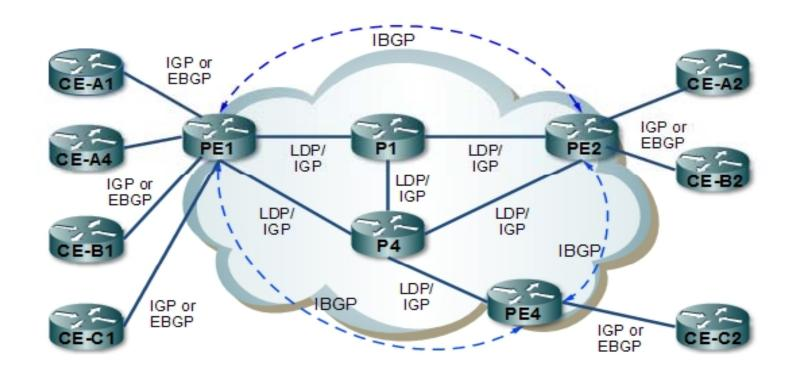
• P routers provide label switching between provider edge routers and are unaware of VPN routes.
